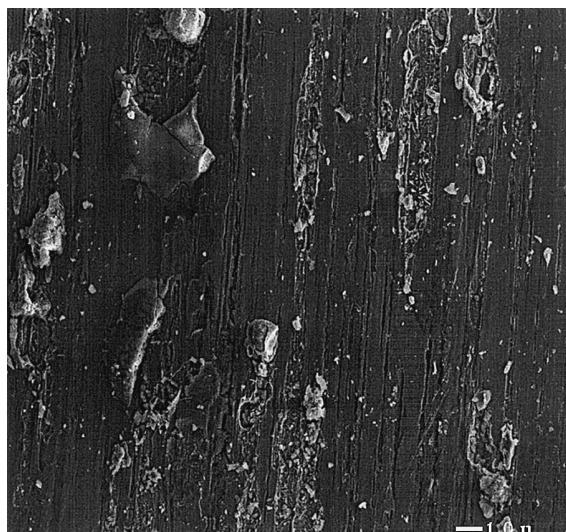
Fig. 11. SEM photograph of surface of untreated coupon after iodine adsorption in air and desorption in air.
